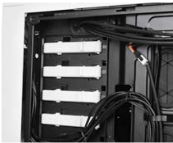
Tool-free design for 5.25" device
