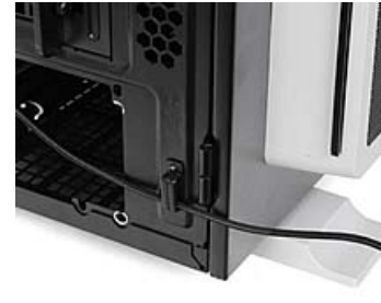
Keyboard & mouse security lock
