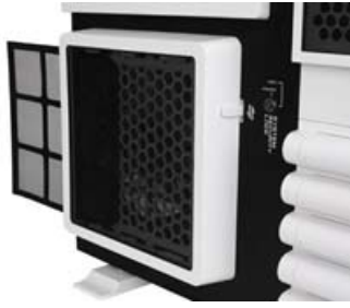
Removable side fan filter
